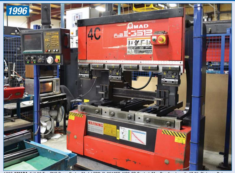
1996 **AMADA** 4' X 38 Ton CNC Press Brake, Model FBD-III-3512FS, NC9-FS Control, Max Bending Length 47.2", Distance Between Housings 40.2", Throat Depth 15.75", Stroke 5.91", Open Height 16.54", 460V, sn 35120130 [4C] (Lot 6)
