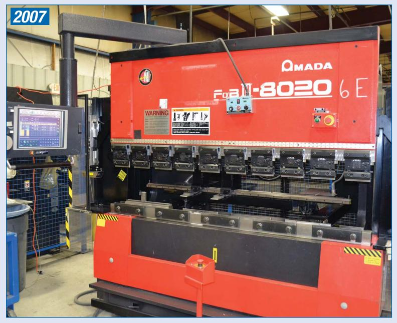
2007 **AMADA** 6.5' x 88 Ton CNC Press Brake, Model FBD-III-8020NT, AMNC PC Control, Max Bending Length 78.7", Distance Between Housings 66.9", Throat Depth 15.75", Stroke 5.91", Open Height 16.54", Laser Safety Lights, 460V, sn 80203133 (Lot 3)
