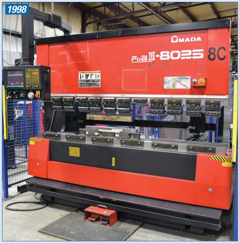
1998 **AMADA** 8' x 88 Ton CNC Press Brake, Model FBD-III-8025FS, NC9-FS Control, Max Bending Length 98.4", Distance Between Housings 86.6" Throat Depth 15.75", Stroke 5.91", Open Height 16.54", Safety Lights, Rear & Side Guarding, 460V, sn 80250609 [8C] (Lot 4) & sn 80250681 [8D] (Lot 5)
